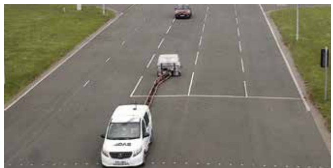
Autonomous Emergency Braking (AEB) testing.
