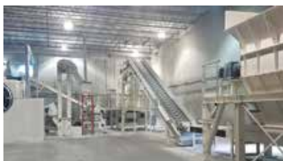
The glass separator used by Safelite's partner, Shark Solutions, to recycle windscreens.
